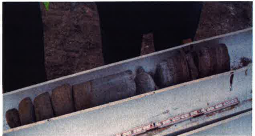
Photo 2 - Clayey Sandstone in B-52 at 10 to 13 feet bgs
