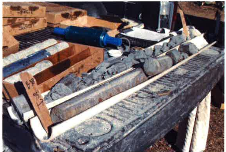
Photo 3 - Clayey Sandstone in B-58 at 95' bgs
